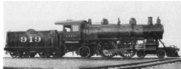
4-4-2 Atlantic type, after 1894 Source: wikipedia under “4-4-2 (locomotive)”
